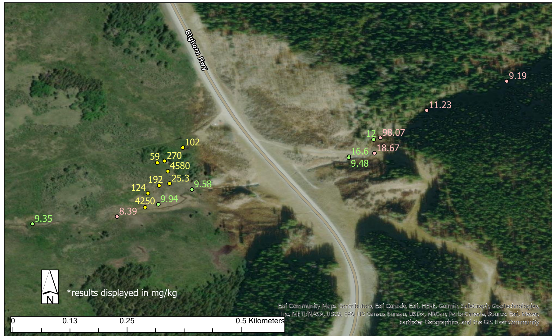
GWAS Lead (Pb) Testing at Four Mile Creek in the Ghost Watershed
